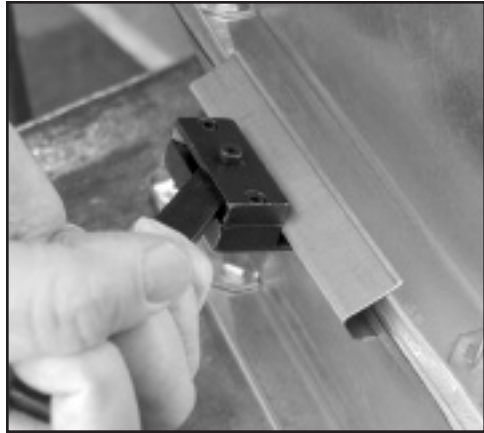
Cleat-Lok™ quickly and easily rolls TDC cleat onto duct joint.
