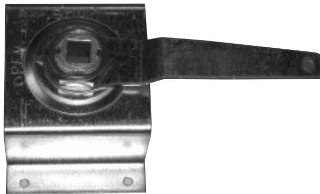
This regulator is designed for insulated duct on low leakage applications. The base is made from 18 gauge galvanized steel. Our Bi-level handle gives extra added elevation to the ductwork. Elevated Regulator Sets for insulated ducts are supplied with a hex nut. These are packaged 25 per carton.
