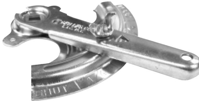
Heavy gauge zinc plated steel quadrant regulators require only twist of a wing nut for easy tightening and adjustments. Base shows damper position. For use with square rod. Stamped handle and base are made from heavy gauge zinc plated steel.
