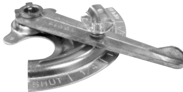
Heavy gauge zinc plated steel quadrant regulators require only a twist of a wing nut for easy tightening and adjustments. Base shows damper position. For use with round rod. Die cast handle made from Zamac #3. Temperature resistant to 728°F and corrosion resistant. The base is made from stamped heavy gauge steel.
