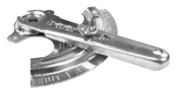
Heavy gauge zinc plated steel quadrant regulators require only twist of a wing nut for easy tightening and adjustments. Base shows damper position. For use with square rod. Stamped handle and base are made from heavy gauge zinc pleated steel.
