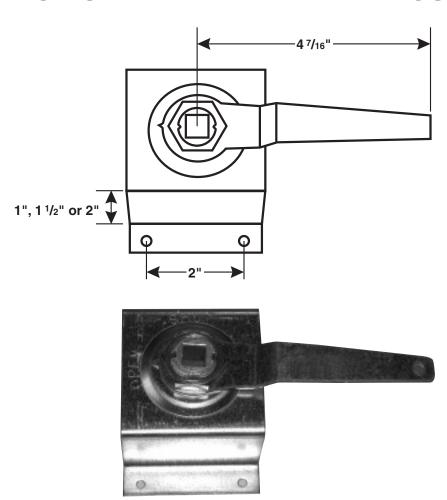
This regulator is designed for insulated duct on low leakage applications. The base is made from 18 gauge galvanized steel. Our Bi-level handle gives extra added elevation to the ductwork. Elevated Regulator Sets for insulated ducts are supplied with a hex nut. These are packaged 25 per carton.
