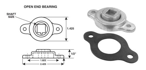
Elgen's Engineered End Bearings are designed for low leakage applications. The regulator is made from a die cast of Zamac #3 (see below) instead of steel. The die cast alloy core is made with serratoins.
