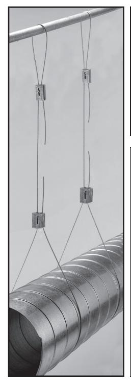
As a matter of sound engineering practice, the Dyna-Tite assembly must be located no closer than 12 inches to the suspension point. In the case of round duct, where the wire rope encircles the duct, the Dyna-Tite must be located the distance of one diameter from the duct wall.
