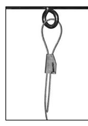
2. Loop Cable through eye bolt and into locking mechanism of clutcher.
