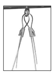
4. Loop Cable through the same eye bolt as in step 2 and secure with a second Clutcher using same method as steps 1 and 2.
