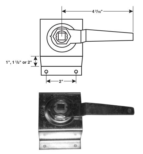
This regulator is designed for insulated duct on low leakage applications. The base is made from 18 gauge galvanized steel. Our Bi-level handle gives extra added elevation to the ductwork. Elevated Regulator Sets for insulated ducts are supplied with a hex nut. These are packaged 25 per carton.
