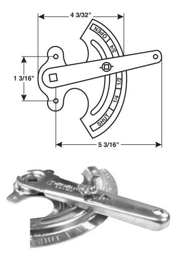
Heavy gauge zinc plated steel quadrant regulators require only twist of a wing nut for easy tightening and adjustments. Base shows damper position. For use with square rod. Stamped handle and base are made from heavy gauge zinc pleated steel.
