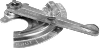
Heavy gauge zinc plated steel quadrant regulators require only a twist of a wing nut for easy tightening and adjustments. Base shows damper position. For use with round rod. Die cast handle made from Zamac #3. Temperature resistant to 728°F and corrosion resistant. The base is made from stamped heavy gauge steel.
