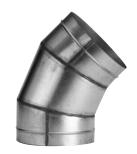
52" and larger in diameter 90 degree full sweep (1.5 x CL) elbows are fabricated using two 45 degree angles connected with an E-Z flange and barrel clamp unless otherwise specified.
