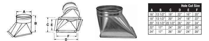
Our High-Efficiency Takeoff is designed with a rectangular opening and an approximate 45° slope on the body. A flange is turned out on all four sides. The flange also has pre-punched holes for easy installation. There is a closed cell neoprene gasket (<sup>3</sup>/4" X <sup>1</sup>/4") applied to the flange to assure a tight seal.
